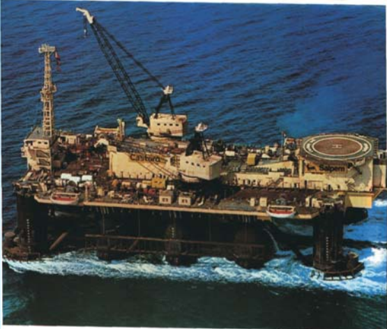
Length overall 151.80 m / Breadth moulded 70.50 m Depth to main deck 29.80 m / Maximum draft 15.50 m Full displacement 41,500 tons / Accommodation for 270 persons
